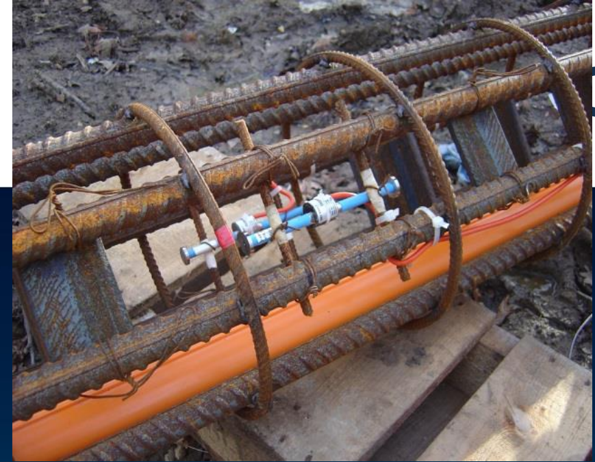
Strain gauges fixed to pile reinforcement cage
